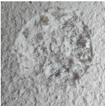
Fig. 4. A representative pull-off fracture image of the composite material coated on aluminum substrate. Other replicates show the same features.
