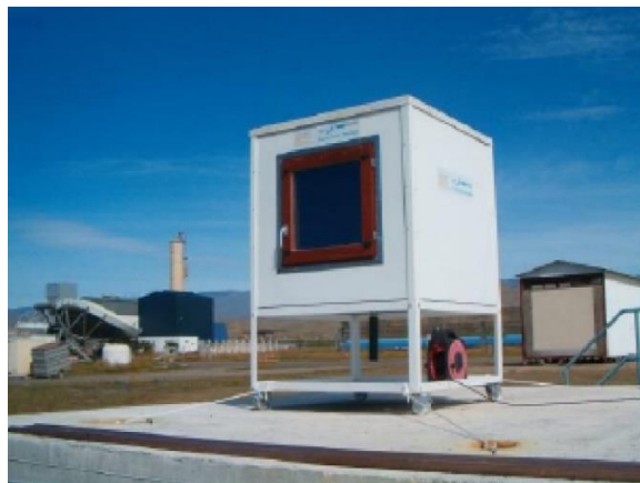
Figure 2. Picture of the Round Robin box set up at the CIEMAT test site
