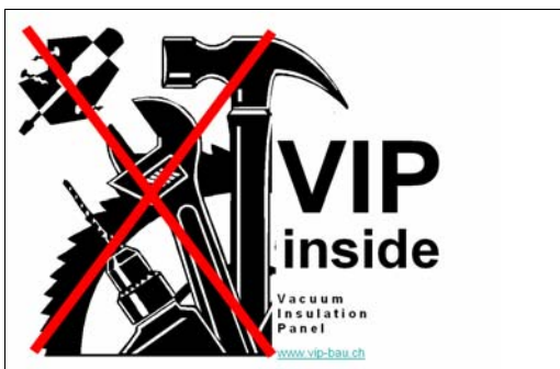
Figure 17: Draft sketch for an adhesive warning label to mark VIP panels and building components containing VIP.
