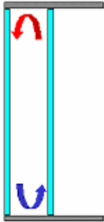
Figure 2.4. DSF - buffer configuration
