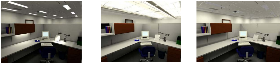
Figure 10-22. Example of computer-generated images of various lighting schemes for cubicles tested to identify preferences among observers.
