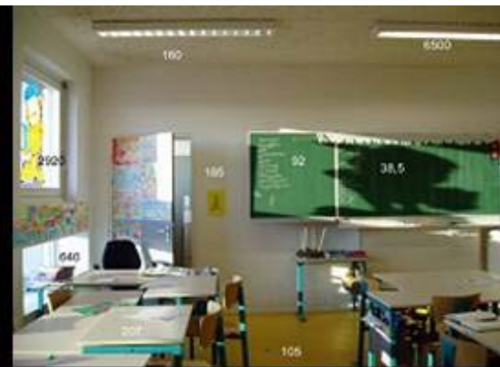
Figure 10 -70. Luminance measurements in south classroom.
