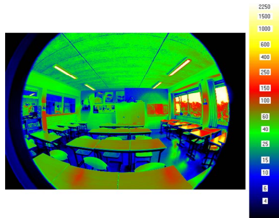
Figure10 -61. Classroom2.20with electricallighting,seenfromteacher position.
