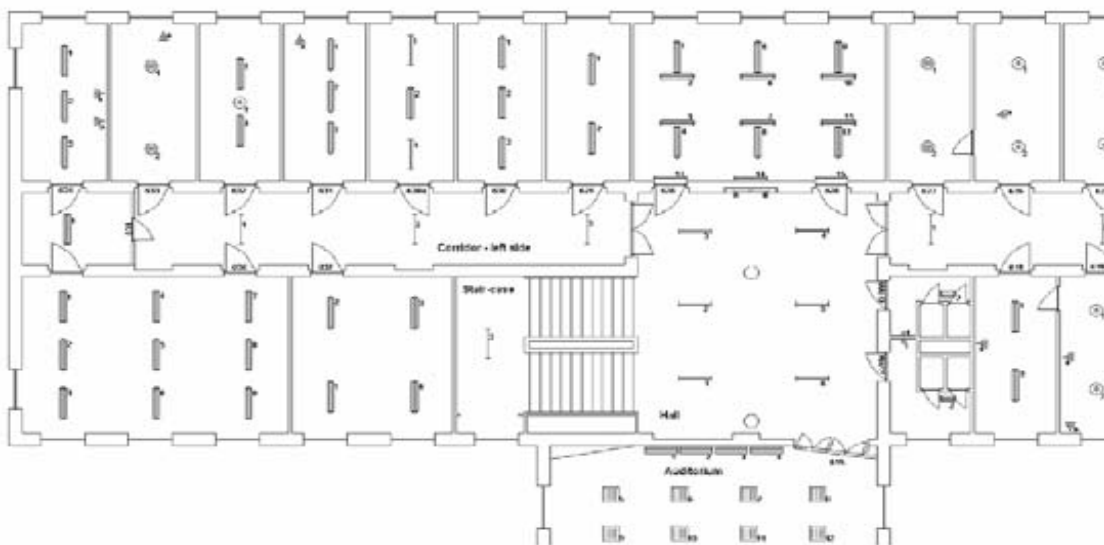
Figure 10.91 Luminaire placement (half of the 3rd floor).
