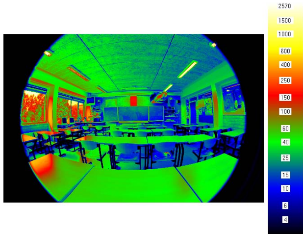
Figure 10 -55. Classroom 2.23 with electrical lighting, seen from student position.
