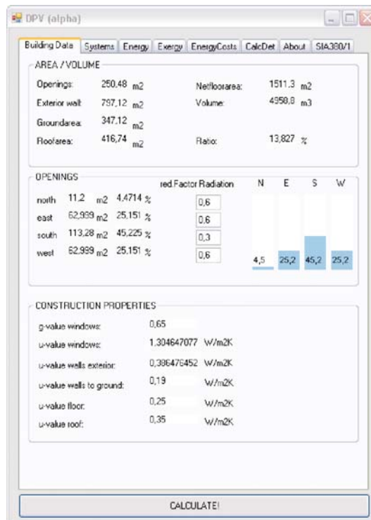
Figure 3.18: Building Data tab of the DPV software showing the calculations made for the building geometry taken from the BIM software.
