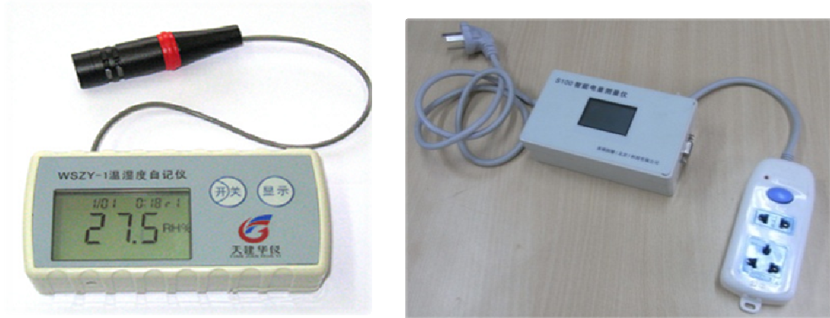
Figure 18-6. The meters are distributed in each room and monitor all the electrical appliances.
