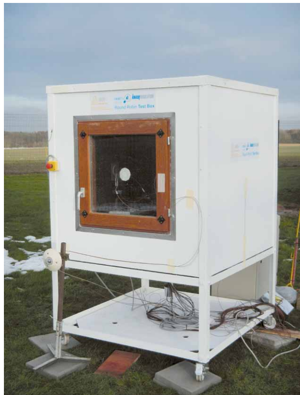
Round robin test box used for in situ characterisation under different climatic conditions.
