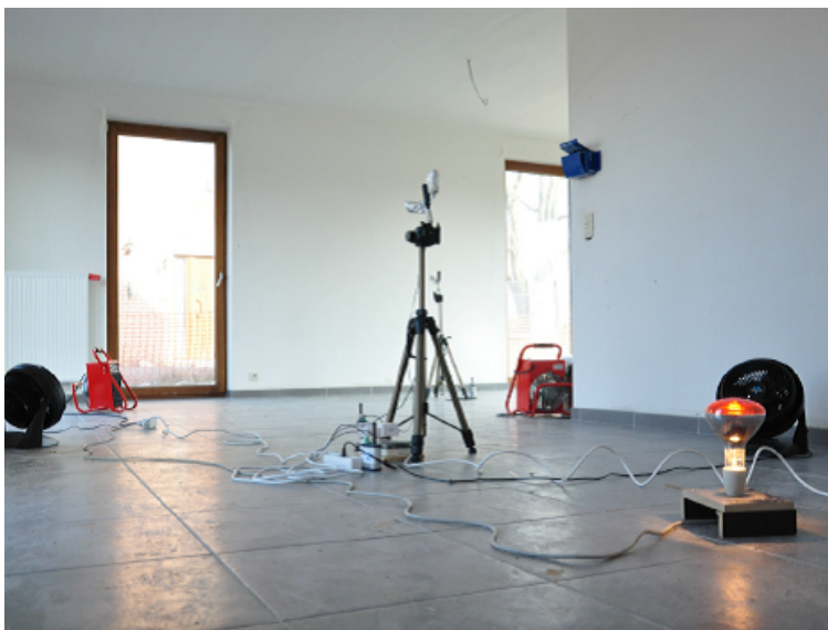
Figure 1: Onsite assessment of thermal performance of the building fabric of a newly built dwelling making use of rather intrusive tests in an unoccupied building (Bauwens G, 2015).
